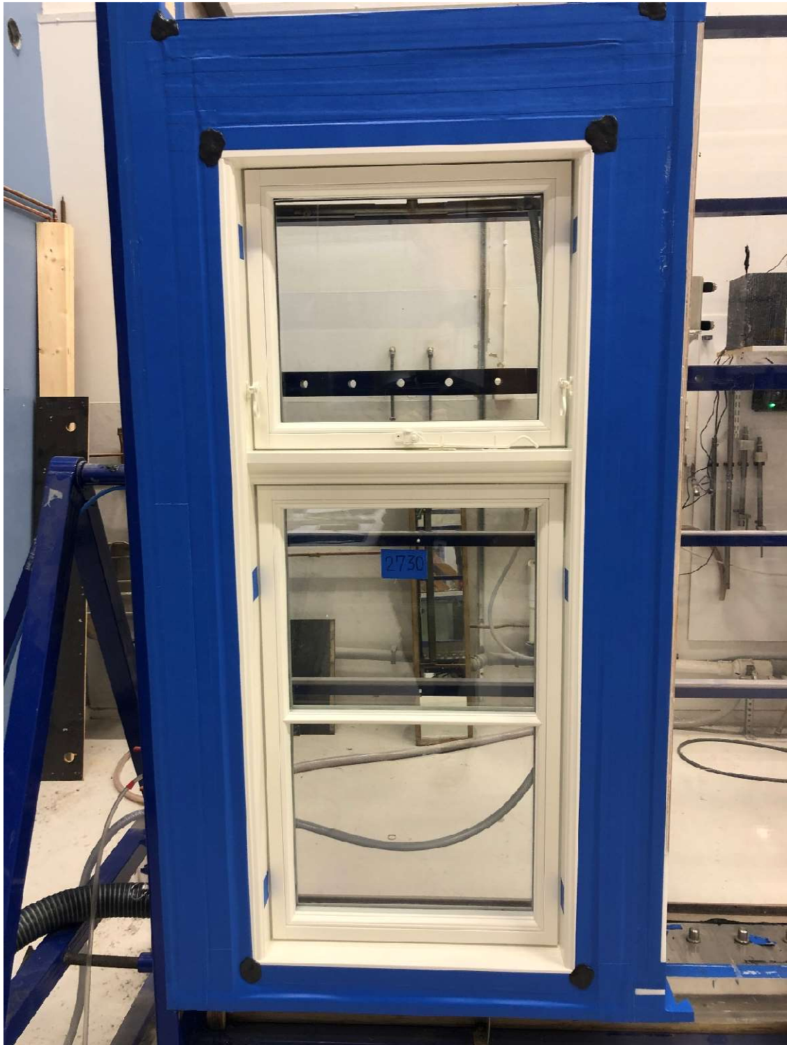
Figure 1: Inside face of the test object mounted in the test rig. Air tightening on inside face.
